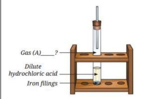
**Answer:** By analysing the figure, it is found that there will be a chemical reaction inside the test tube between dilute HCl and Fe.
